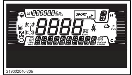
The MODE display indicates the selected mode of operation:
