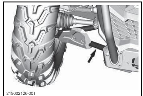
5. Firmly attach the rear suspension tie-down straps to both sides of the rear of the trailer with ratchets.
