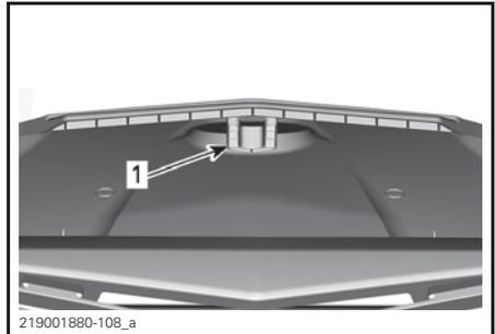
1. Locating slot on underside of service cover
