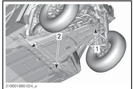
1. Lifting location under skid plate
