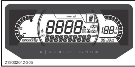
This display shows gears position of gearbox:
