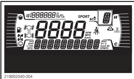
This display shows gear position of gearbox:
