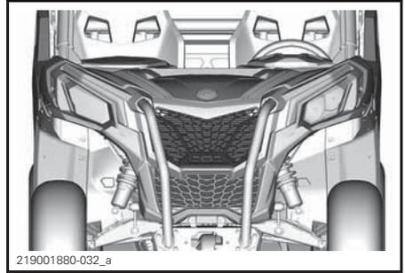
Inspect radiator and hoses for leaks or any damage.
