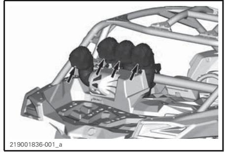
Remove air filter cap to let out any water that may have been introduced.
