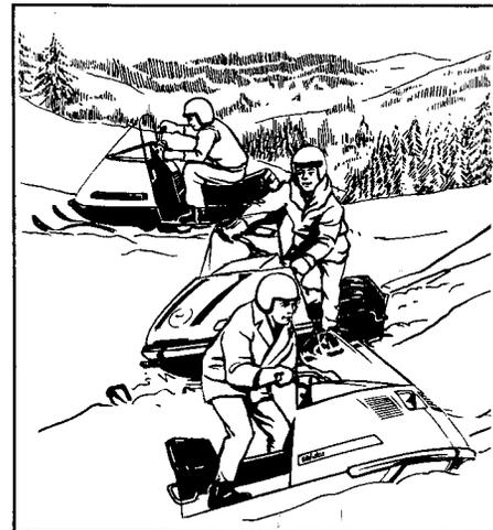
of the fun of snowmobiling is that each turn depends on 4 factors — the radius of the turn, vehicle speed, snow conditions and the weight on the skis.
