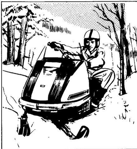
**Icy Surface** — Ice or extremely hard-packed snow can be difficult to negotiate as both skis and track do not have much traction. Best advice is to slow down and avoid rapid acceleration or braking.
