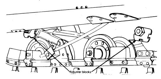
CAUTION: Always turn left side adjuster blocks in a clockwise direction, the right side blocks in a counter-clockwise direction. Left and right adjuster blocks of each adjustment must always be set at the same elevation.
