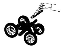
Grease each set then spray the springs with metal protector, or wipe with an oil soaked cloth. Assemble and install each set in the proper position.
