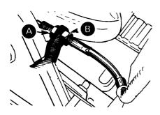
Once minor adjustment is completed, firmly tighten the nuts (A and B) against the bracket. If correct brake control lever clearance is unobtainable, proceed with major adjustment as follows:
