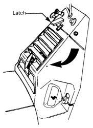
2. Push the console downward then tilt away from the engine. To reinstall, reverse the procedure.
