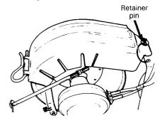
To remove the drive pulley guard, pull out the retaining clip (A) and pull on the spring (B) to disengage the pin from the bracket.
