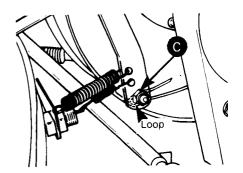
WARNING: Brake cable must make a loop around the bolt head. Strongly pull the brake handle to check cable tightness. Always check the brake light to see if it functions after performing brake adjustment.
