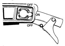
WARNING: For safety reasons, the emergency cut-off switch is easily accessible; be careful not to operate it inadvertently.
