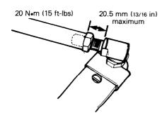
Handlebar should also be horizontal when the skis are pointed toward the front. To adjust; loosen the lock nuts of the shorter tie rod. Turn the tie rod manually until the handlebar is horizontal. Retighten the lock nuts firmly. Check tightness of the steering arm locking bolts and the wear of the ball joints.
