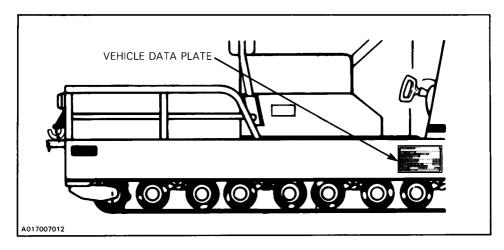
The vehicle data plate appears on the right hand side of the chassis, as shown.
