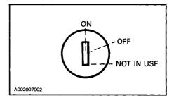
Key operated, 3 position switch. To start engine, first turn key fully clockwise to START position and hold. Return key to ON position immediately when engine has started. To stop engine, turn key counterclockwise to OFF position. The 3rd position is not in use.
