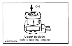
Ensure the tether cut-out cap is in position and that the cord is attached to your clothing.
