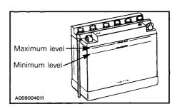
If necessary add distilled water. Battery connections must also be free of corrosion. If cleaning is necessary remove corrosion using a stiff brush then clean with a solution of baking soda and water. Rinse and dry well.
