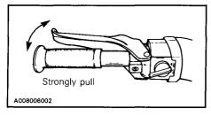
After the adjustment, brake should apply fully when lever is approximatively 13 mm (1/2'') from handlebar grip. If not, do not tamper with the brake, contact your authorized dealer
