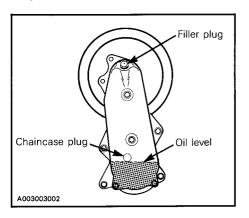
The oil should be level with the bottom of the oil level orifice. Refill as required using Bombardier chaincase oil (P/N 413 8019 00 - 200 ml).
