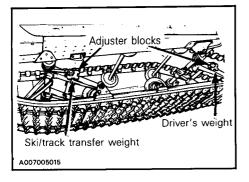
When the front adjuster blocks are at the lowest elevation more weight is distributed on the skis.
