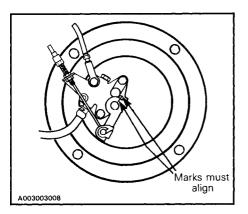
CAUTION: The carburetor must be adjusted before adjusting the oil injection pump. Make sure the idle speed is 1100-1300 R.P.M.
