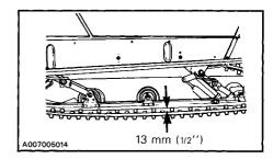
CAUTION: Too much tension will result in power loss and excessive stresses on suspension components.
