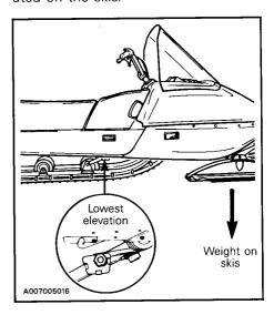
At the highest position the weight is transferred from the skis to the track. The rear adjuster blocks should be adjusted to suit the driver's preference.
