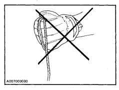
WARNING: When starting the vehicle in an emergency situation by the drive pulley, do not make a knot at the end of the emergency rope and do do not reinstall the belt guard.
