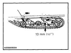
CAUTION: Too much tension will result in power loss and excessive stresses on suspension components.
