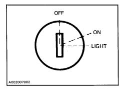
Key operated 3 position switch. To start engine, first turn key clockwise to ON position. To stop engine, turn key counterclockwise to OFF position.
