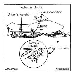
When the front adjuster blocks are at the lowest elevation more weight is distributed on the skis.
