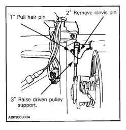
3. Open the driven pulley by twisting and pushing the sliding half. Hold in fully open position.
