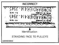
CAUTION: Do not force or use tools to pry the belt into place, as this could cut or break the cords in the belt.
