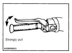
After the adjustment, brake should apply fully when lever is approximatively 13 mm (1/2") from handlebar grip. If not, do not tamper with the brake, contact the dealer.
