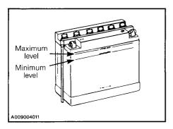
If necessary add distilled water. Battery connections must also be free of corrosion. If cleaning is necessary remove corrosion using a stiff brush then clean with a solution of baking soda and water. Rinse and dry well.
