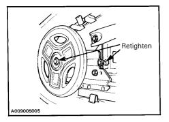
Restart engine, rotate track **slowly** and recheck alignment.
