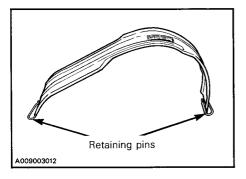
3. Lift and remove the belt guard assembly.
