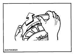
4. Slip slackened belt over the top edge of the sliding half.
