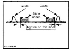
Tighten lock nuts and the idler wheel retaining screws.
