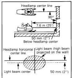
To adjust, remove the four caps, turn upper or lower adjusting screws to obtain desired beam position.
