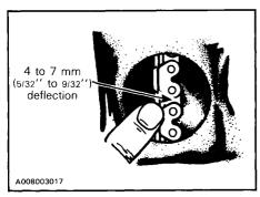
To adjust, loosen lock nut and turn adjuster bolt to obtain the specified freeplay. Tighten lock nut and recheck chain tension
