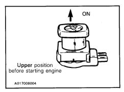
Ensure the tether cut-out cap is in position and that the cord is attached to your clothing.
