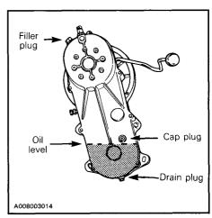
NOTE: Drain plug is accessible through a hole located underneath vehicle.
