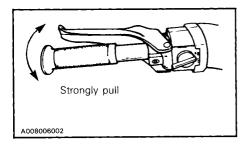
After the adjustment, brake should apply fully when lever is approximatively 13 mm (1/2'') from handlebar grip. If not, do not tamper with the brake, contact an authorized dealer.
