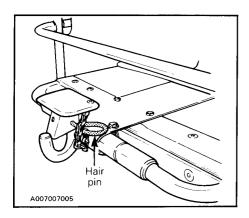
Fixed on the rear bumper. A hair pin is supplied to lock the hook attachment.
