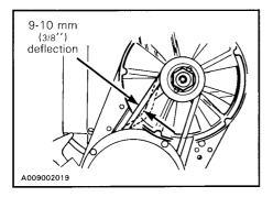
If belt seems damaged or if tension is incorrect, contact the dealer immediately.
