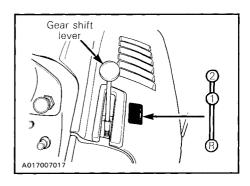
WARNING: This snowmobile is capable of a fast reverse. On first outing, operator should become familiar with this operation by practicing on level ground. Always apply the brake before shifting and come to a complete stop then, while holding brake on, change gear. This is particularly important while on a slope. Ensure the path behing is clear of obstacles or bystanders. Fast reverse, while turning, could result in loss of stability.
