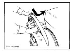
Slip slackened belt over the top edge of the driven pulley sliding half, opposite side of gearbox.
