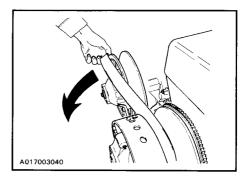
4. Completely remove the belt from the driven pulley and lie flat under the driven pulley outside edge.
