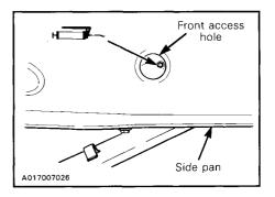
CAUTION: Ensure to lubricate both drive axles. A grease fitting is located on each side pan.
