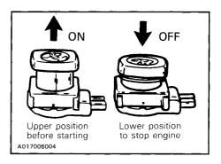
WARNING: For safety reasons, the emergency cut-out switch is easily accessible; be careful not to operate it inadvertently.
