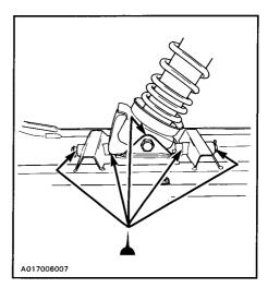
Allow the oil to run in and move ski several times to distribute lubricant.
