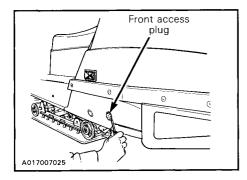
Lubricate at grease fitting using low temperature grease then reinstall access plug.
