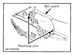
3. Lift and remove the belt guard.
