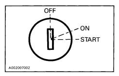
Key operated, 3 position switch. To start engine, turn key to START position and hold. Return key to ON position immediately when engine has started. To stop engine, turn key to OFF position. If engine does not start on first try, key must be turned fully back to OFF each time.
