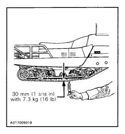
CAUTION: Too much tension will result in power loss and excessive stresses on suspension components.
