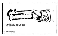
After the adjustment, brake should apply fully when lever is approximatively 13 mm (1/2") from handlebar grip. If not, do not tamper with the brake, contact an authorized dealer.
