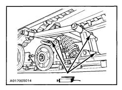
Coat inside of stabilizer bar bushing of rear suspension with grease.
