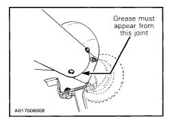
Oil tie rod ball joints and steering column upper and lower bushings.
