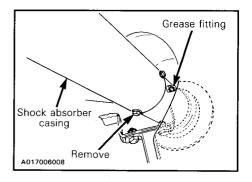
Lubricate until the grease appears from the hole, then, firmly plug the hole with a finger and slowly continue to lubricate until grease appears at the joint.
