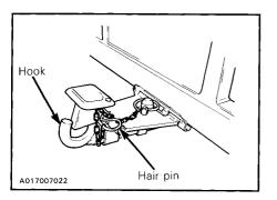
WARNING: When towing any sled or trailer, always ensure to lock the hook type attachment with the hair pin.
