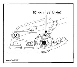
NOTE: For deep snow or hill climbing, it is recommended to place the front adjuster blocks on the lowest position and set stopper strap to the shortest position.
