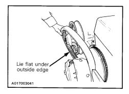
5. Slip belt out from the drive pulley and remove completely from the vehicle.
