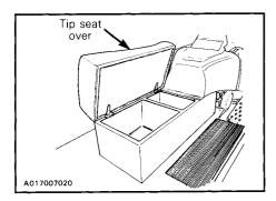
NOTE: Emergency materials should be wrapped in foam or similar material. This will prevent possible damage to breakable items when travailling over rought or bumpy terrain.
