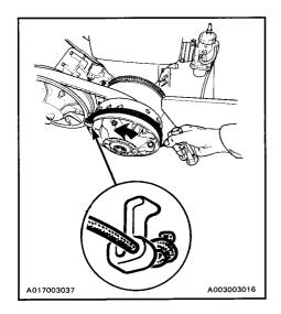
Start engine as per usual manual starting. Reinstall console but not belt guard.
