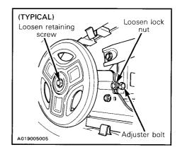
NOTE: Track tension and alignment are inter-related. Do not adjust one without the other.
