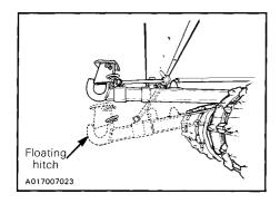
The locking pin can be installed into hair pin when the hitch is used floating.
