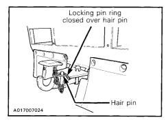
NOTE: To maintain the hitch locked, install the locking pin into hitch post and place its flat side against the hitch plate.
