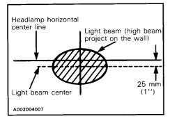
To adjust, remove the four (4) caps, turn upper or lower adjusting screws to obtain desired beam position.
