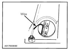
To fill, remove filler cap from top of gearbox. Refill as required using Bombardier chaincase oil (P/N 413 8019 00, 250 ml).
