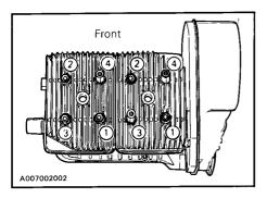
**IMPORTANT**: The engine head nut torque should be checked after the first five (5) hours of operation.
