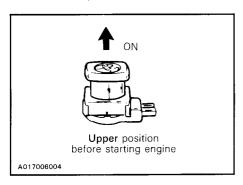
Ensure the tether cut-out cap is in position and that the cord is attached to the clothing.
