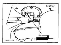
CAUTION: When lubricating the drive axle bearing, do not apply excessive grease as the seal will be pushed out of its housing. Check seal position with finger.
