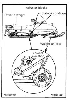
When the front adjuster blocks are at the lowest elevation more weight is distributed on the skis.
