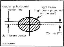
To adjust, remove the four (4) caps, turn upper or lower adjusting screws to obtain desired beam position.
