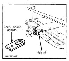
WARNING: When towing a sled or trailer, always ensure to lock the hook with the hair pin.
