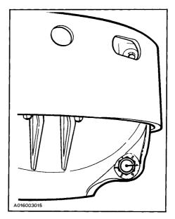
CAUTION: Back off the calibration screw locking nut only far enough to allow a change of position of the screw head. **Never** attempt to remove the locking nut or the calibration screw. Make sure the adjustment is set at the **same** position for all three (3) screws.
