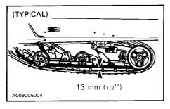
CAUTION: Too much tension will result in power loss and excessive stresses on suspension components.
