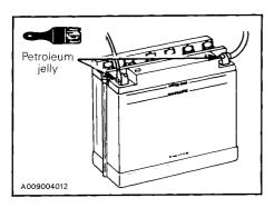
WARNING: Vent tube must be free and open. If not, it will restrict ventilation and create a gas accumulation that could result in an explosion. Avoid skin contact with electrolyte.
