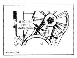
If belt seems damaged or if tension is incorrect, contact an authorized dealer immediately.
