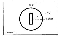
Key operated 3 position switch. To start engine, first turn key to ON position. To stop engine, turn key to OFF position.
