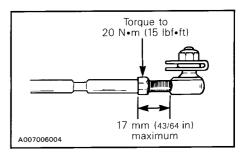
WARNING: The ball joint socket must run parallel with the steering arm. The tie rod must be restrained when tightening the tie rod end lock nuts.
