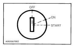
Key operated, 3 position switch. To start engine, turn key to START position and hold. Return key to ON position immediately when engine has started. To stop engine, turn key to OFF position.
