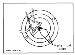
CAUTION: The carburetor must be adjusted before adjusting the oil injection pump. Make sure the idle speed is 1100-1300 R.P.M.
