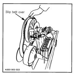
5. Slip the belt out from the drive pulley and remove completely from vehicle.
