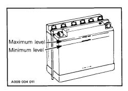
If necessary add distilled water. Battery connections must also be free of corrosion. If cleaning is necessary remove corrosion using a stiff brush then clean with a solution of baking soda and water. Rinse and dry well.
