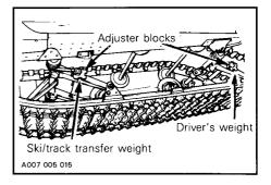
When the front adjuster blocks are at the lowest elevation more weight is distributed on the skis
