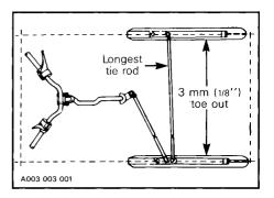
The handlebar should also be horizontal when the skis are pointed toward the front.
