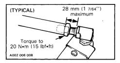
WARNING: The ball joint socket must run parallel with the steering arm. The tie rod must be restrained when tightening the tie rod end lock nuts.
