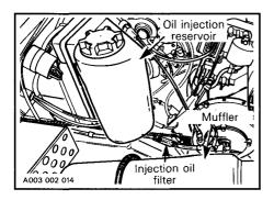
CAUTION: An obstructed injection oil filter will cause oil starvation resulting in serious engine damage.
