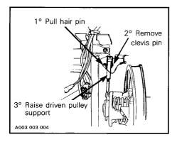
Open the driven pulley by twisting and pushing the sliding half. Hold in fully open position.
