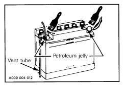
WARNING: Vent tube must be free and open. If not, it will restrict ventilation and create a gas accumulation that could result in an explosion. Avoid skin contact with electrolyte.
