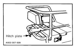
The vehicle is equipped with a hitch, plate type, on the rear bumper. A hook type may be fitted to the actual hitch. Consult your authorized dealer for details.
