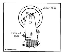
The oil should be level with the bottom of the oil level orifice. Refill as required using Bombardier chaincase oil (P/N 413 8019 00 - 250 ml (9 oz)).
