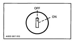
Key operated, 2 position switch. To start engine, first turn key to ON position. To stop engine, turn key to OFF position.
