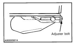
NOTE: Track tension and alignment are inter-related. Do not adjust one without checking the other.
