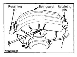
To remove the pulley guard, pull out the retaining clip (A) and pull on the spring (B) to disengage the pin from the bracket.
