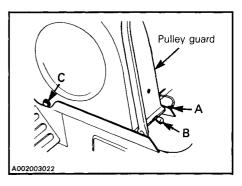
Push the pulley guard forward to disengage the front attachment (C) from the frame. Lift the guard from the vehicle.
