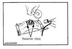
If taillight bulb is burnt, remove the red plastic lens and replace bulb.
