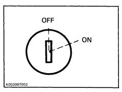
Key operated, 2 position switch. To start the engine, first turn the key to ON position. To stop the engine, turn the key to OFF position.
