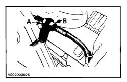
Once minor adjustment is completed, firmly tighten the nuts (A and B) against the bracket. If correct brake control lever clearance is unobtainable, proceed with major adjustment as follows:
