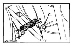
WARNING: Brake cable must make a loop around the bolt head. Strongly pull the brake handle to check cable tightness. Always check the brake light to see if it functions after performing brake adjustment.
