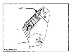
Push the console downward then tilt away from the engine. To reinstall, reverse the procedure.
