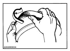
4. Slip the belt out from the drive pulley and remove completely from the vehicle. To install the drive belt, reverse the procedure, however pay attention to the following.
