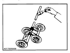
Grease each bogie wheel until the old grease is flushed out. Spray bogie wheel springs with metal protector. If unavailable, wipe with a cloth or rag soaked in oil.
