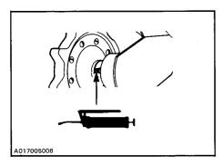
CAUTION:When lubricating the rear axle bearing, do not apply excessive grease as the seal will be pushed out of its housing. Check seal position with finger.
