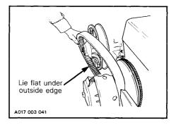
5. Slip belt out from the drive pulley and remove completely from the vehicle.
