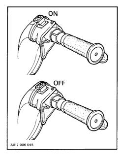
WARNING: For safety reasons, the emergency cut-out switch is easily accessible; be careful not to operate it inadvertently. If the switch has been used in an emergency situation the source of malfunction should be determined and corrected before restarting engine.
