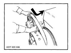
Slip slackened belt over the top edge of the driven pulley sliding half, opposite side of gearbox.
