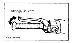
After the adjustment, brake should apply fully when lever is approximatively 13 mm (1/2 in) from handlebar grip. If not, do not tamper with the brake, contact an authorized dealer.
