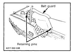
3. Lift and remove the belt guard.
