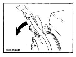
Completely remove the belt from the driven pulley and lie flat under the driven pulley outside edge.
