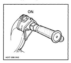
Ensure the tether cut-out cap is in position and that the cord is attached to your clothing.
