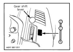
WARNING: This snowmobile is capable of a fast reverse. Operator should become familiar with this operation by practicing on level ground. Always apply the brake before shifting and come to a complete stop then, while holding brake on, change gear. Ensure the path behing is clear of obstacles or bystanders. Fast reverse, while turning, could result in loss of stability.
