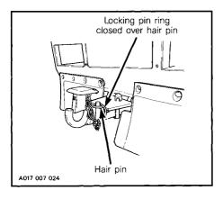
NOTE: To maintain the hitch locked, install the locking pin into hitch post and place its flat side against the hitch plate.
