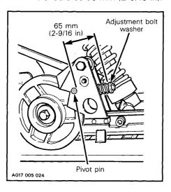
NOTE: The driver can customize this adjustment to meet its particular need. For instance should one is most of the time pulling a load and use rarely the reverse, the rear pivot could be "locked" by fully tighten the adjustment bolt thus getting a better traction and a more positive steering.
