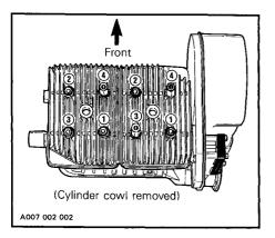
IMPORTANT: The engine head nut torque should be checked after the first 5 hours of operation.
