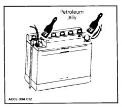
WARNING: Vent tube must be free and open. If not, it will restrict ventilation and create a gas accumulation that could result in an explosion. Avoid skin contact with electrolyte. Gases given off by a battery being charged are highly explosive. Always charge in a well ventilated area. Keep battery away from cigarettes or open flames. Avoid skin contact with electrolyte.
