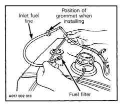
Replace fuel filter. To facilitate the fuel line installation, slide grommet on fuel line about 50 mm (2 in) away from elbow than install grommet on fuel tank and push down elbow through grommet.
