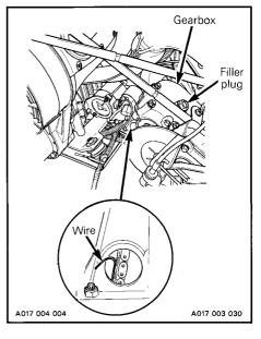
To fill, remove filler plug from top of gearbox. Refill as required using Bombardier chaincase oil (P/N 413 8019 00, 250 mL (9 oz)).
