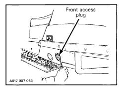
Lubricate using low temperature grease then reinstall access plugs.
