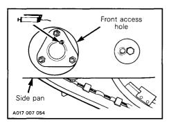
CAUTION: Ensure to lubricate both drive axles. A grease fitting is located on each side pan.
