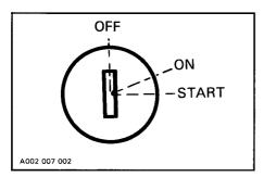
Key operated, 3 position switch. To start engine, turn key to START position and hold. Return key to ON position immediately when engine has started. To stop engine, turn key to OFF position. If engine does not start on first try, key must be turned fully back to OFF each time.
