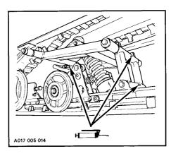
Coat inside of stabilizer bar bushing of rear suspension with grease.
