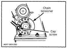
Rotate the tensioner as required to obtain correct chain tension.
