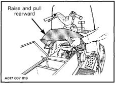
When installing console to vehicle, ensure to insert console tabs into dashboard slots.
