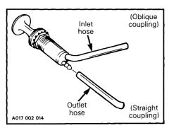
6. Insert storage oil (P/N 496 0141 00) can hose into primer outlet hose.
