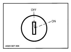
Key operated two position switch. To start the engine, first turn key to ON position. To stop engine, turn key to OFF position.
