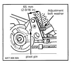
NOTE: The driver can customize this adjustment to meet its particular need. For instance should one is most of the time pulling a load and use rarely the reverse, the rear pivot could be "locked" by fully tighten the adjustment bolt thus getting a better traction and a more positive steering.
