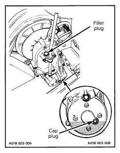
To fill, remove filler plug from top of transmission. Refill as required using Bombardier chaincase oil (P/N 413 8019 00 - 250 ml).
