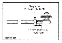
WARNING: The ball joint socket must run parallel with the steering arm. The tie rod must be restrained when tightening the tie rod end lock nuts.
