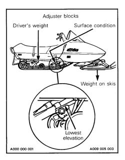
When the front adjuster blocks are at the lowest elevation more weight is distributed on the skis.
