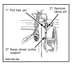
3. Open the driven pulley by twisting and pushing the sliding half. Hold in fully open position.
