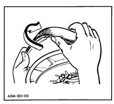
5. Slip the belt out from the drive pulley and remove completely from vehicle.
