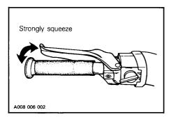
After the adjustment, brake should apply fully when lever is approximatively 13 mm (1/2 in) from handlebar grip. If not, do not tamper with the brake, contact the dealer.
