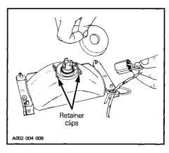
If taillight bulb is burnt, expose the bulb by removing the red plastic lens. To remove, unfasten the two (2) screws.
