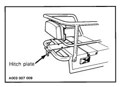
The Safari Cheyenne is equipped with a hitch, plate, on the rear bumper. A hook type may be fitted to the actual hitch. Consult your authorized dealer for details.
