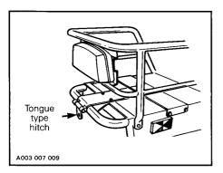
The vehicle is equipped with a tongue type hitch, on the rear bumper. A hook type may be fitted to the actual hitch. Consult your authorized dealer for details.
