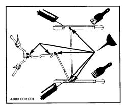
Oil spring coupler bolts, ball joints and steering column bushings.
