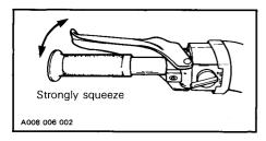
After the adjustment, brake should apply fully when lever is approximatively 13 mm (1/2 in) from handlebar grip. If not, do not tamper with the brake, contact your authorized dealer.
