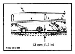
CAUTION: Too much tension will result in power loss and excessive stresses on suspension components.
