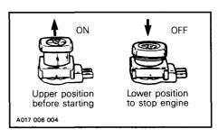
WARNING: For safety reasons, the emergency cut-off switch is easily accessible; be careful not to operate it inadvertently. If the switch has been used in an emergency situation the source of malfunction should be determined and corrected before restarting engine.
