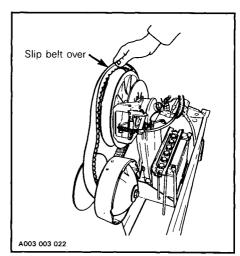
5. Slip the belt out from the drive pulley and remove completely from vehicle.
