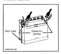
WARNING: Vent tube must be free and open. If not, it will restrict ventilation and create a gas accumulation that could result in an explosion. Avoid skin contact with electrolyte. Gases given off by a battery being charged are highly explosive. Always charge in a well ventilated area. Keep battery away from cigarettes or open flames. Avoid skin contact with electrolyte.
