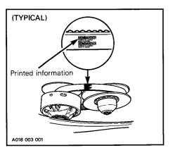
CAUTION: Do not force or use tools to pry the belt into place, as this could cut or break the cords in the belt.
