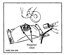
If taillight bulb is burnt, expose the bulb by removing the red plastic lens. To remove, unfasten the two screws.
