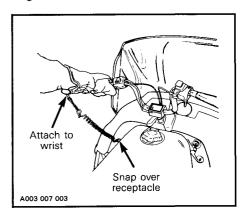
If emergency engine "shut off" is required, completely pull cap from safety switch and engine power will be automatically shut "off".
