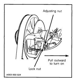
Tighten the lock nut while restraining the other one. Recheck brake light operation.
