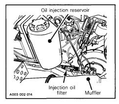
CAUTION: An obstructed injection oil filter will cause oil starvation resulting in serious engine damage.
