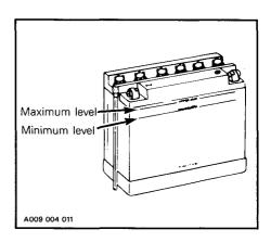
If necessary add distilled water. Battery connections must also be free of corrosion. If cleaning is necessary remove corrosion using a stiff brush then clean with a solution of baking soda and water. Rinse and dry well.
