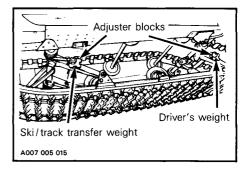
When the front adjuster blocks are at the lowest elevation more weight is distributed on the skis.
