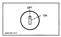
Key operated, two position switch. To start engine, first turn key to ON position. To stop engine, turn key to OFF position.
