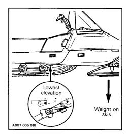
At the highest position the weight is transferred from the skis to the track. The rear adjuster blocks should be adjusted to suit the driver's preference.
