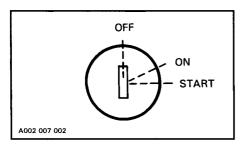
Key operated, three position switch. To start engine, turn key to START position and hold. Return key to ON position immediately when engine has started. To stop engine, turn key to OFF position.
