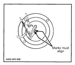
CAUTION: The carburetor must be adjusted before adjusting the oil injection pump. Make sure the idle speed is 1800-2000 RPM.
