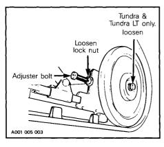
NOTE: Track tension and alignment are inter-related. Do not adjust one without the other.
