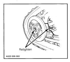
Restart engine, rotate track **slowly** and recheck alignment.
