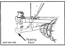
The locking pin can be installed into hair pin when the hitch is used floating.
