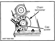
Rotate the tensioner as required to obtain correct chain tension.
