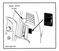
WARNING: This snowmobile is capable of a fast reverse. Operator should become familiar with this operation by practicing on level ground. Always apply the brake before shifting and come to a complete stop then, while holding brake on, change gear. Ensure the path behing is clear of obstacles or bystanders. Fast reverse, while turning, could result in loss of stability.
