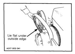
6. Slip belt out from the drive pulley and remove completely from the vehicle.
