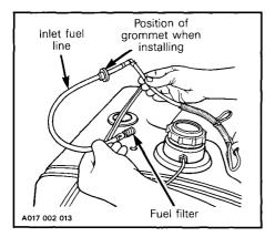
Replace fuel filter. To facilitate the fuel line installation, slide grommet on fuel line about 50 mm (2 in) away from elbow than install grommet on fuel tank and push down elbow through grommet.
