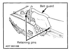
3. Lift and remove the belt guard.
