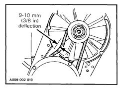
If belt seems damaged or if tension is incorrect, contact the dealer immediately.
