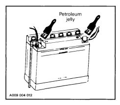
WARNING: Vent tube must be free and open. If not, it will restrict ventilation and create a gas accumulation that could result in an explosion. Avoid skin contact with electrolyte. Gases given off by a battery being charged are highly explosive. Always charge in a well ventilated area. Keep battery away from cigarettes or open flames.
