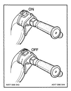
WARNING: If the switch has been used in an emergency situation the source of malfunction should be determined and corrected before restarting engine.
