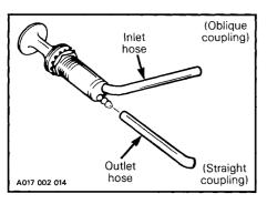
Insert storage oil (P/N 496 0141 00) can hose into primer outlet hose.
