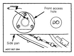
CAUTION: Ensure to lubricate both drive axles. A grease fitting is located on each side pan.
