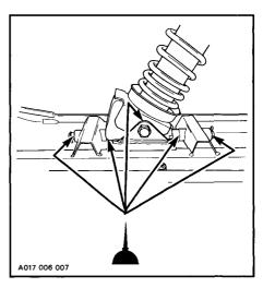
Allow the oil to run in and move ski several times to distribute lubricant.
