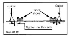
Tighten lock nuts and the idler wheel retaining screws.
