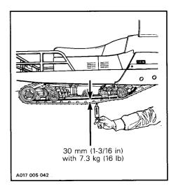
CAUTION: Too much tension will result in power loss and excessive stresses on suspension components.
