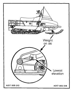
At the highest position, the weight is transferred to the track thus giving a better traction to pull a load.
