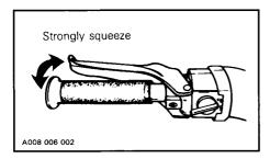
After the adjustment, brake should apply fully when lever is approximatively 13 mm (1/2 in) from handlebar grip. If not, do not tamper with the brake, contact an authorized dealer.
