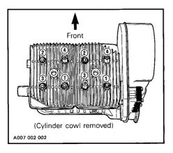
IMPORTANT: The engine head nut torque should be checked after the first 5 hours of operation.
