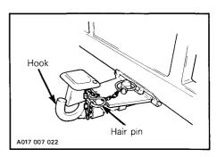
WARNING: When towing any sled or trailer, always ensure to lock the hook type attachment with the hair pin.
