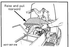
When installing console to vehicle, ensure to insert console tabs into dashboard slots
