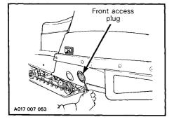
Lubricate using low temperature grease then reinstall access plugs.
