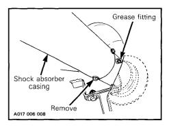
Lubricate until the grease appears from the hole, then, firmly plug the hole with a finger and slowly continue to lubricate until grease appears at the joint.
