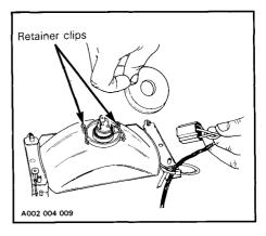
If taillight bulb is burnt, remove the red plastic lens and replace bulb.
