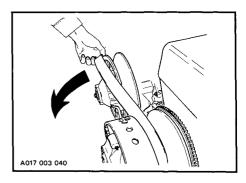
5. Completely remove the belt from the driven pulley and lie flat under the driven pulley outside edge.
