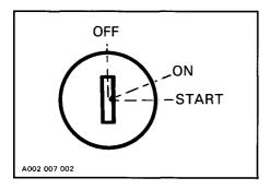
Key operated, three position switch. To start engine, turn key to START position and hold. Return key to ON position immediately when engine has started. To stop engine, turn key to OFF position. If engine does not start on first try, key must be turned fully back to OFF each time.
