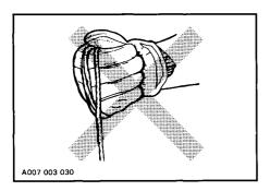
WARNING: Do not start the vehicle by the drive pulley unless it is a true emergency situation. Have the vehicle repaired as soon as possible.
