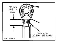
WARNING: The ball joint socket must run parallel with the steering arm and the other ball joint. The socket must be restrained when tightening the tie rod end lock nuts.
