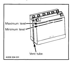
If necessary add distilled water. Battery connections must also be free of corrosion. If cleaning is necessary remove corrosion using a stiff brush then clean with a solution of baking soda and water. Rinse and dry well.
