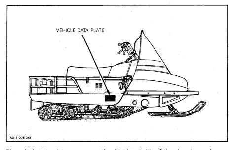
The vehicle data plate appears on the right hand side of the chassis, as shown.
