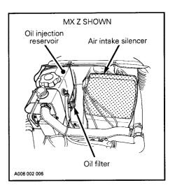
CAUTION: An obstructed injection oil filter will cause oil starvation resulting in serious engine damage.
