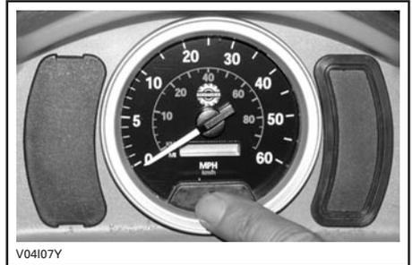
The odometer can indicate **in miles or in kilometers**. See an authorized Bombardier ATV dealer to change the indications.
