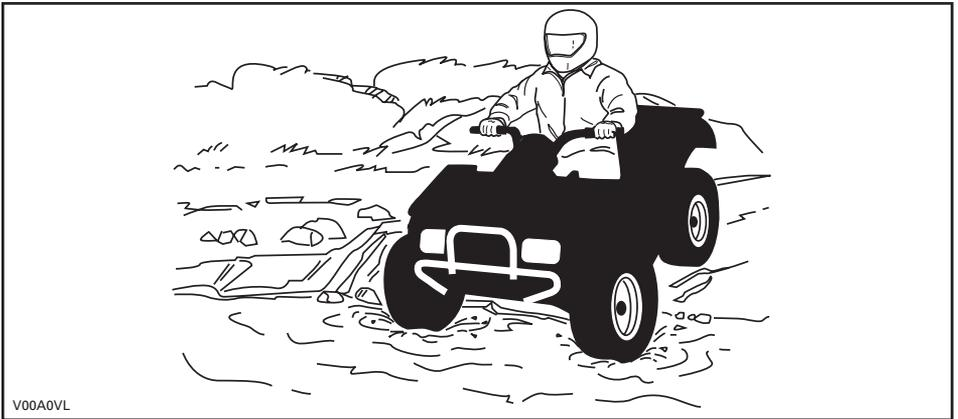
Water will affect the braking ability of your vehicle. Make sure you dry the brakes by applying them several times after the vehicle leaves the water.
