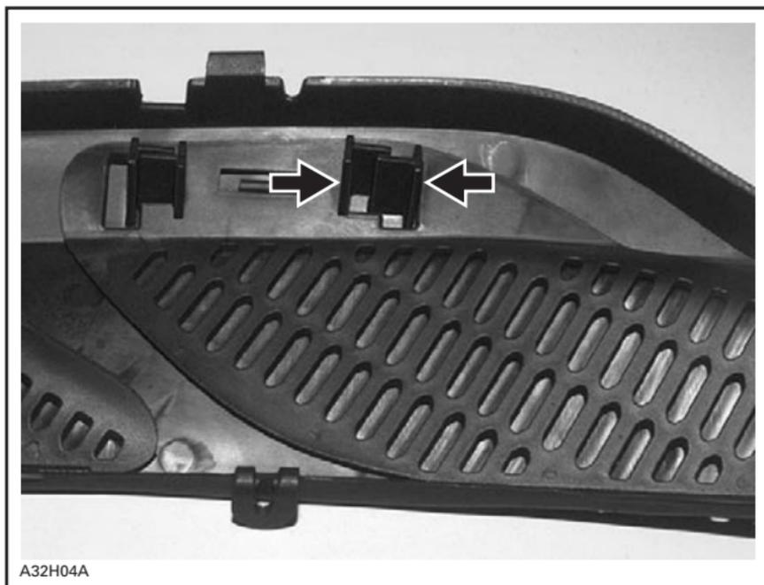
*TO OPEN, SQUEEZE OPENING TABS BETWEEN THUMB AND INDEX*
