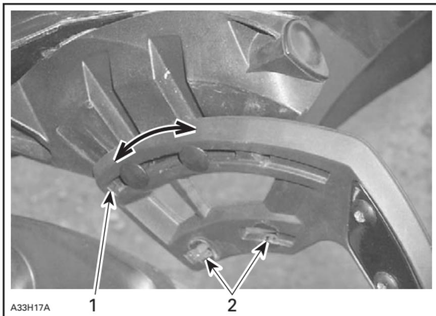
1. Slot when windshield is installed for rearward steering column position
