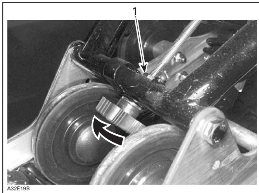
1. Loosen lock nut, turn knob accordingly then retighten lock nut
