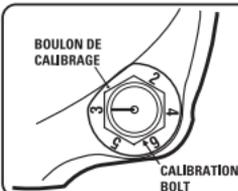
Adjust all three drive pulley bolts to same position.
