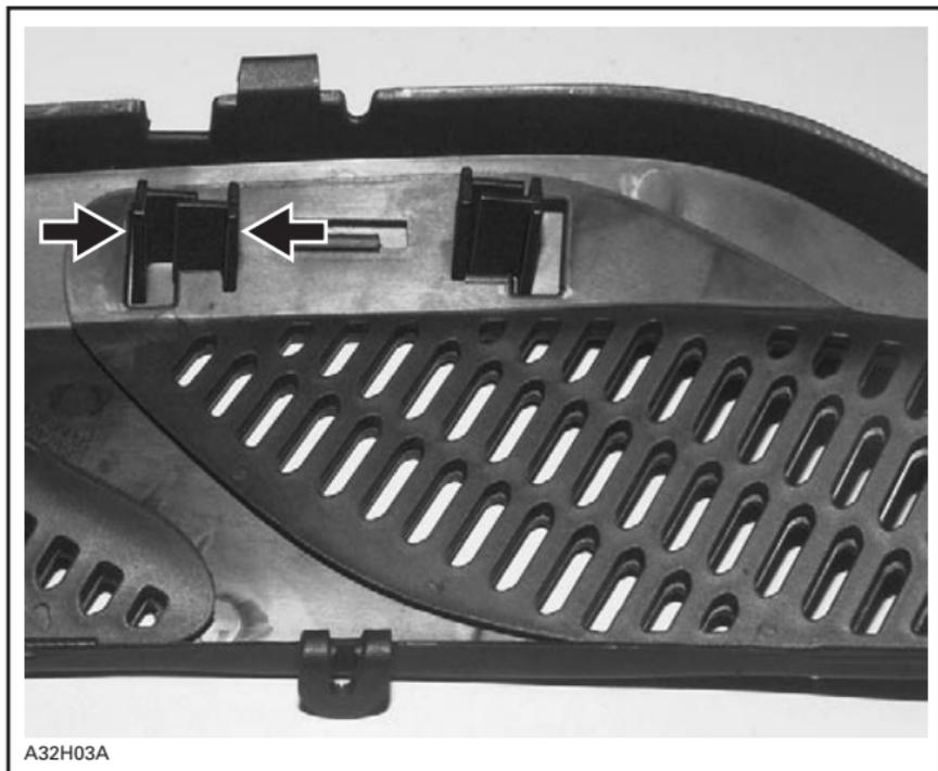
*TO CLOSE, SQUEEZE CLOSING TABS BETWEEN THUMB AND INDEX*
