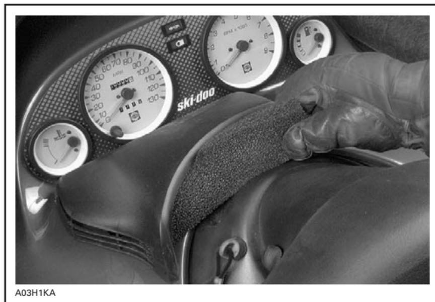
**TYPICAL — REMOVING FILTER**
