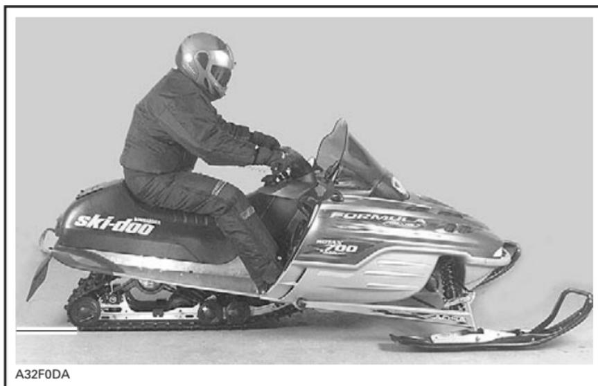
**TYPICAL** — **TOO HARD OF ADJUSTMENT** (REAR SUSPENSION RUNS TOO HIGH, IT HAS COLLAPSED LESS THAN 50 mm (2 in))
