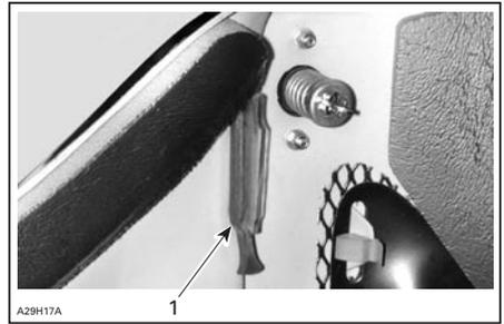
1. One of the top two latches temporary retaining windshield
