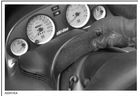
TYPICAL — REMOVING FILTER
