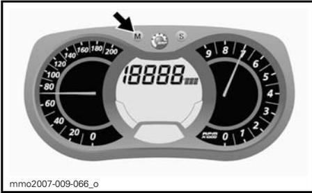
To reset maximum temperature recorded, press the MODE (M) to select mode.
