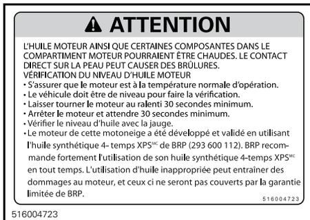
MODÈLE 1200 4-TEC - DANS LE COMPARTIMENT MOTEUR
