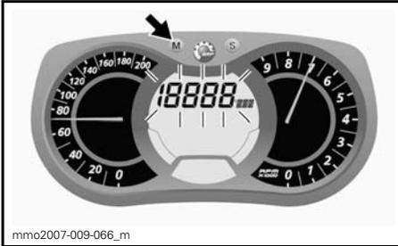
While display flashes, press SET (S) button to select vehicle average speed (AVR\_SPD) mode.
