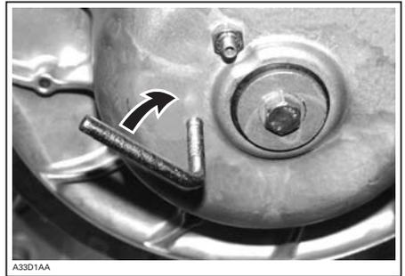
4. Open the driven pulley by screwing the tool in.
