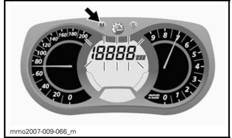
While display is flashing, press the SET (S) button to select speedometer mode.
