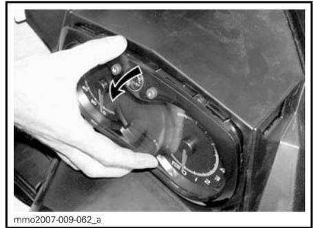
Disconnect burnt bulb connector. Remove the rubber boot.
