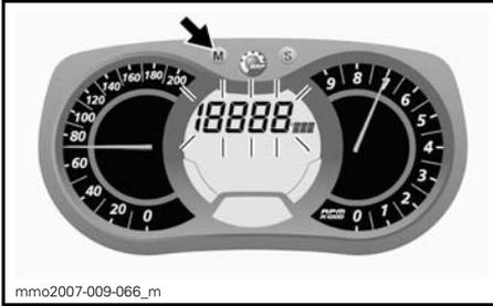
While display flashes, press the SET (S) button to select total fuel consumption (TC) mode.
