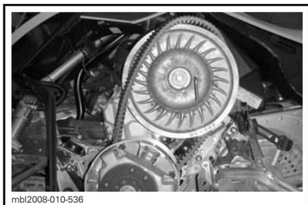
3. Unscrew and remove the drive belt installer/remover tool.
