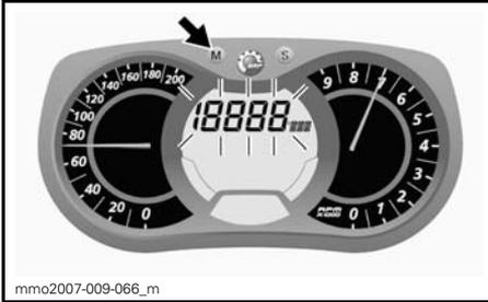
Press and hold the SET (S) button within 5 seconds to reset.
