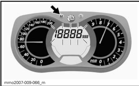
While display flashes, press the SET (S) button to select top speed (TOP\_SPD) mode.
