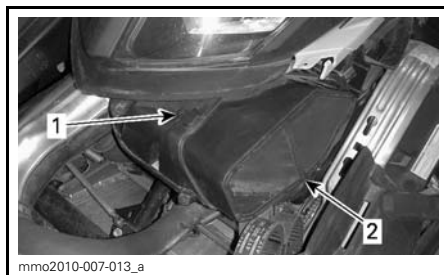
1. Retaining clip 2. Air filter
