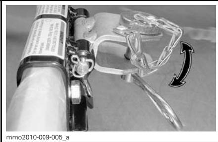
**HITCH MOVES FREELY WHEN TOWING**
