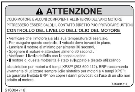
MODELLO 1200 4-TEC - NEL VANO MOTORE
