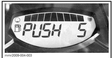
5. When the gauge displays "PUSH S", release all buttons.
