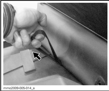
3. Lift up the rear end of seat and gently pull back just enough to expose the accessories connector.
