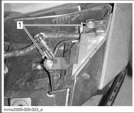
1. *Taillight housing retaining screws*
