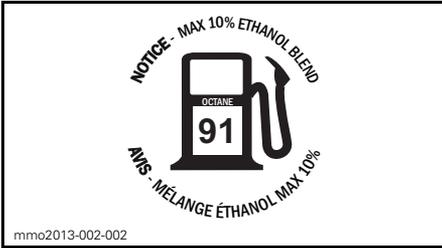
LOCATED ON FUEL CAP - ON E-TEC ENGINES (IN COUNTRIES USING PUMP POSTED AKI (RON+MON)/2 OCTANE RATINGS)
