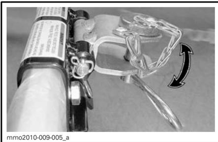
**HITCH MOVES FREELY WHEN TOWING**
