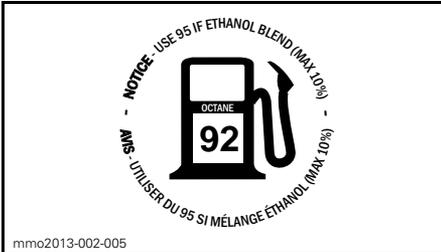
LOCATED ON FUEL CAP - ON 1200 4-TEC AND ACE ENGINES - IN COUNTRIES USING RON OCTANE RATINGS
