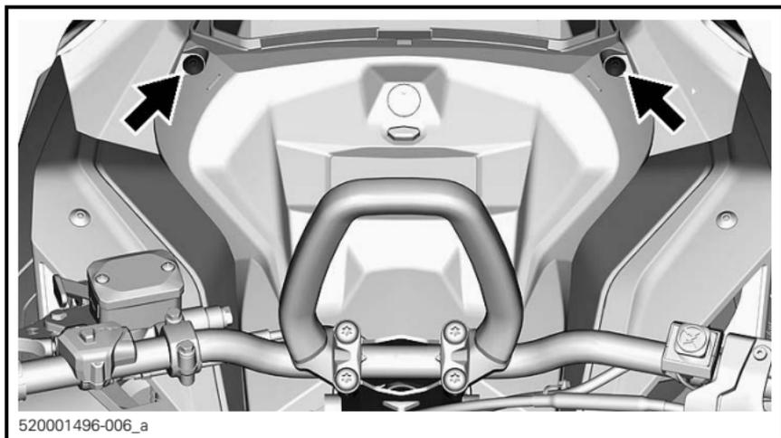
3. Lift the front of the gauge, then slide it forward to remove it.
