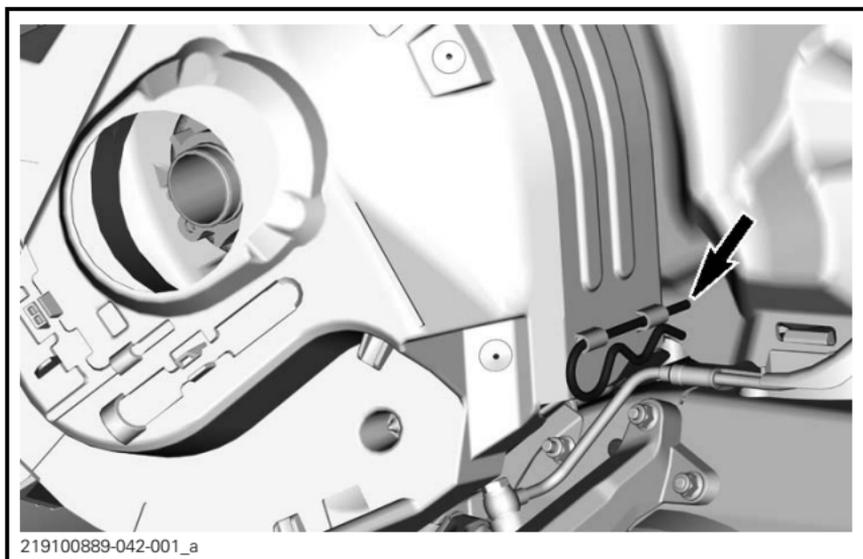
Lift rear portion of guard then release from front tab.
