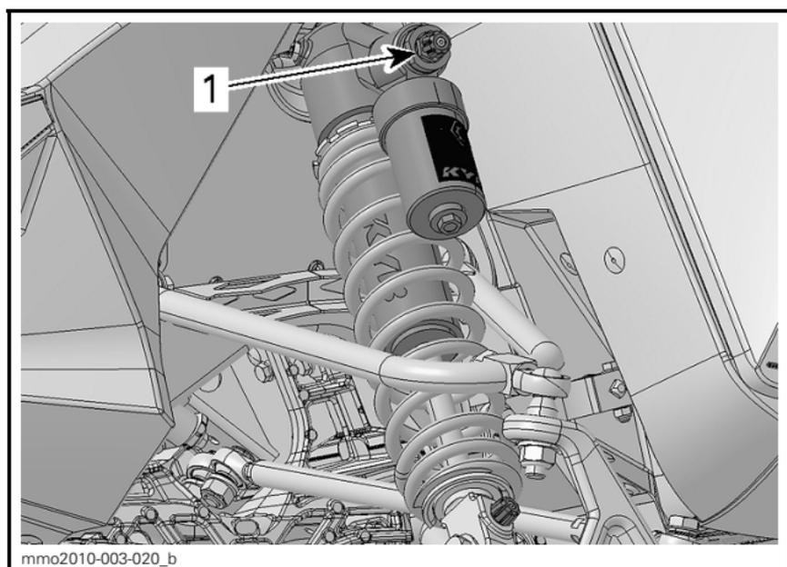
1. High speed compression damping adjuster (hexagonal)
