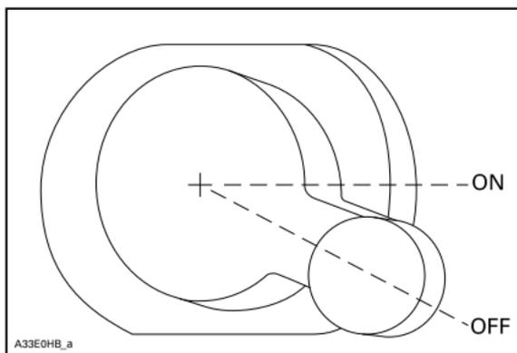
All operators of the snowmobile should familiarize themselves with the function of the emergency engine stop switch by using it several times on first outing and whenever stopping the engine thereafter. This engine stopping procedure will become a reflex and will prepare operators for emergency situations requiring its use.
