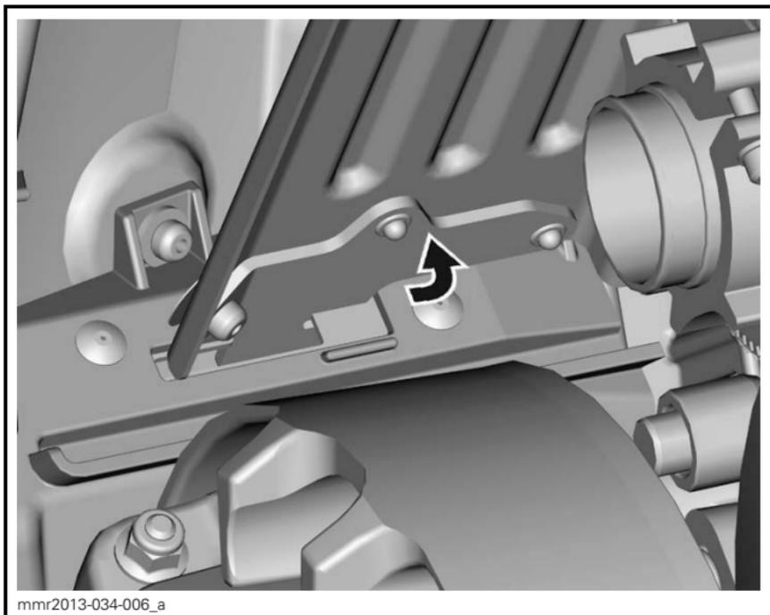
Position the rear portion of the belt guard over the retainer and secure it using the retaining pin.
