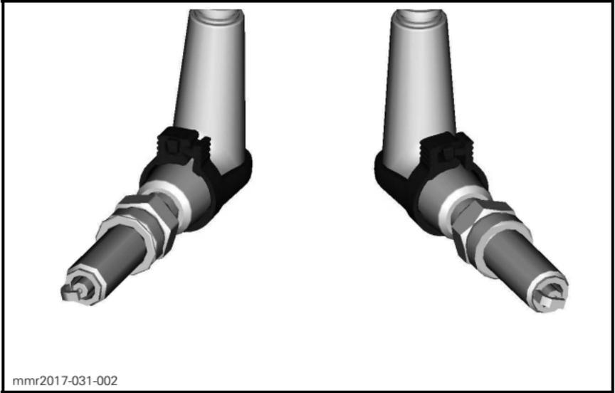
6. Remove spark plug cables as shown.
