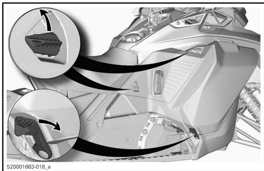
When closing panel, make sure latches are locked securely.
