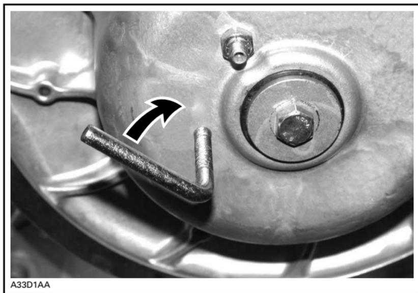
4. Open the driven pulley by screwing the tool in.
