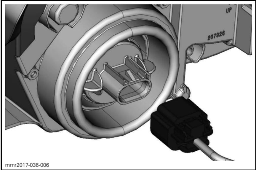
7. Unlock bulb by turning it counterclockwise.
