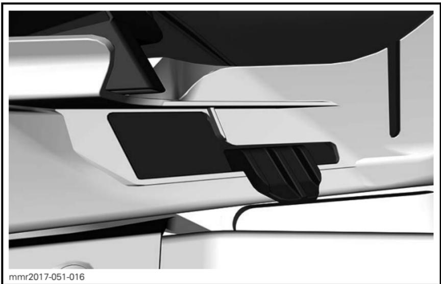
**NOTE:** Make sure the air intake duct is positioned correctly in the boot.
