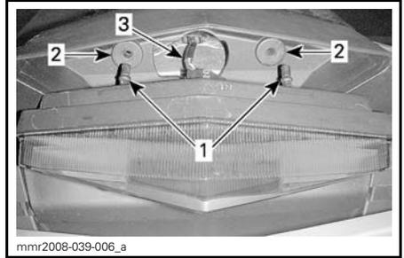
1. Taillight housing retaining pins
