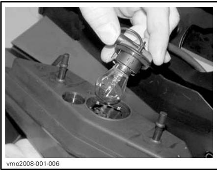
Push the bulb in and hold while turning counterclockwise to release.
