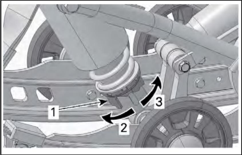
**TYP MIT NOCKE - STOßDÄMPFER MIT EINSTELLBARER DRUCKSTUFENDÄMPFUNG**
