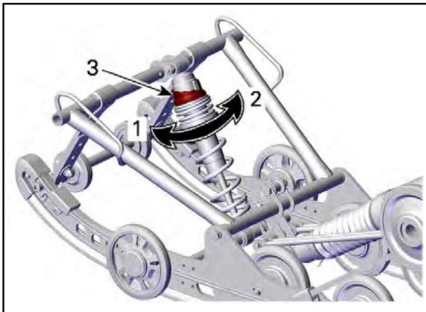
**TYP MIT NOCKEN - HPG-STOßDÄMPFER**
