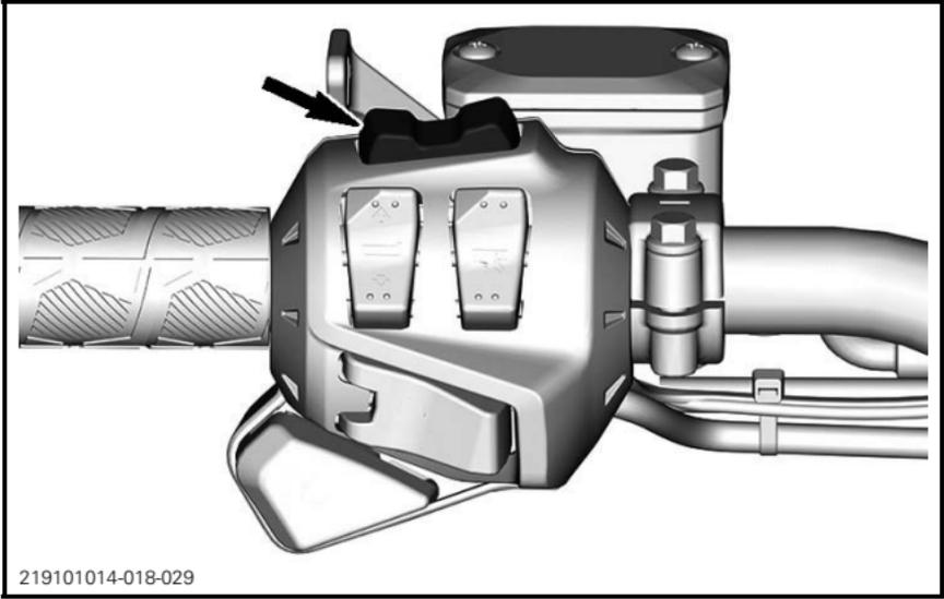
3. Press the MENU (M) button to cycle through suspension settings.
