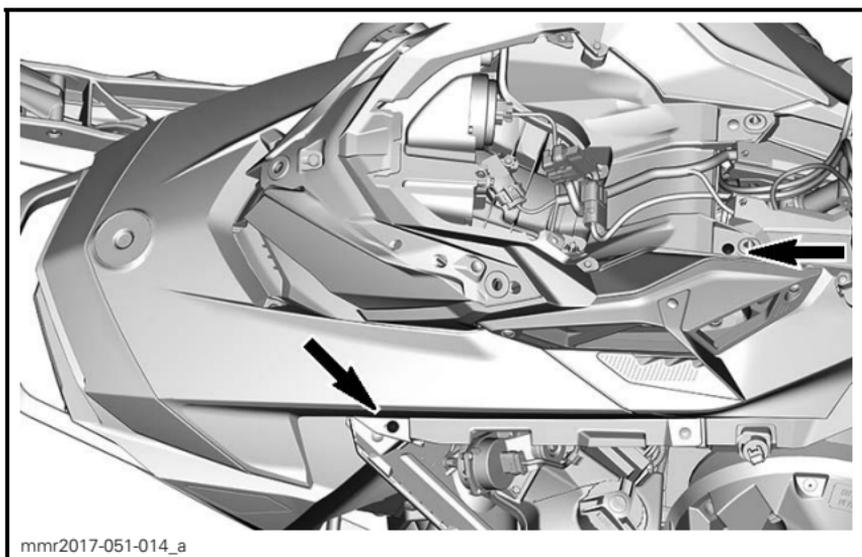
9. Free the rear end hooks of the upper body module from the slots in the console.
