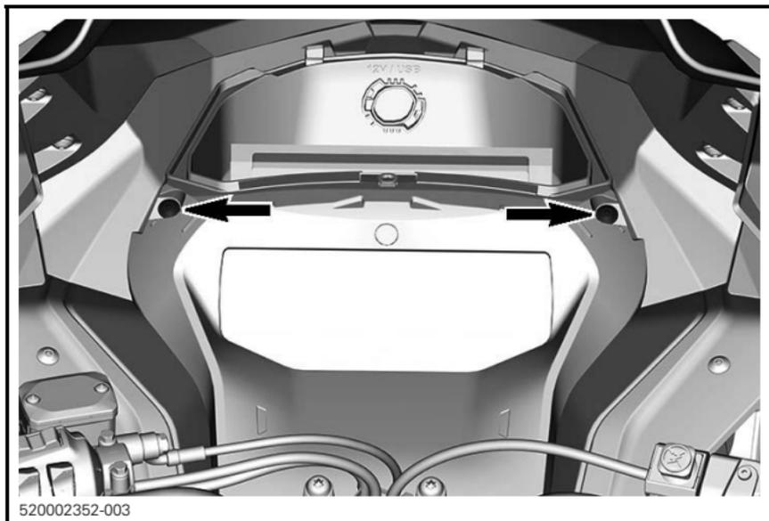
3. Lift the front of the gauge support, then slide it forward to remove it.
