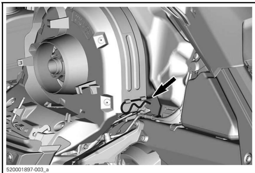
Lift rear portion of guard then release from front tab.
