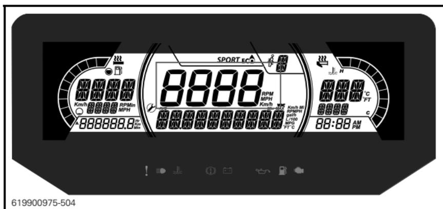
Display the vehicle speed in Km/h (or MPH) or the RPMs. Refer to *SETTINGS*.
