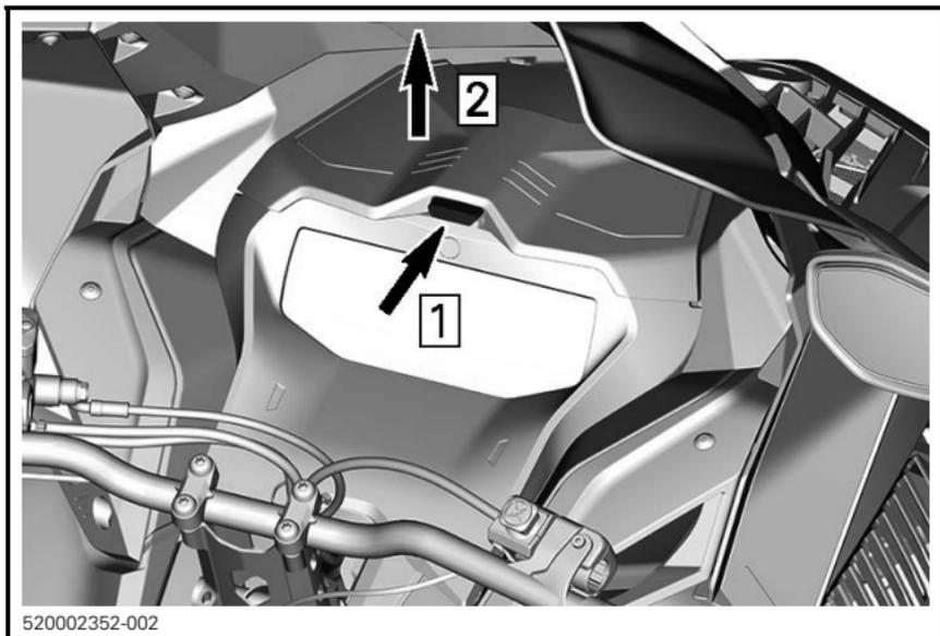
2. Remove the gauge retaining screws.
