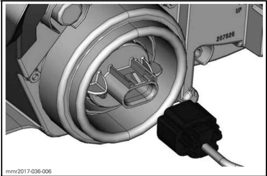
7. Unlock bulb by turning it counterclockwise.
