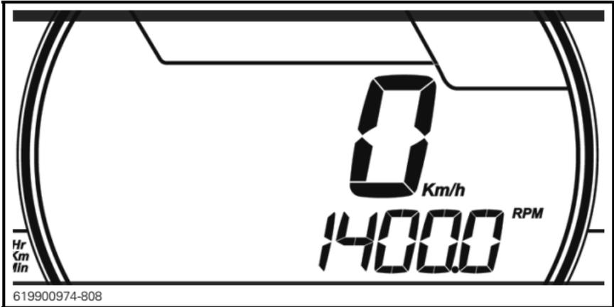
**NOTE:** The storage mode does not function in other modes (trip A, trip B and hr trip).
