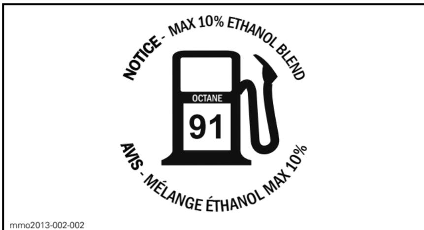
ON FUEL CAP - ON 600R E-TEC AND 850 E-TEC ENGINE IN COUNTRIES USING PUMP POSTED AKI (RON+MON)/2 OCTANE RATINGS
