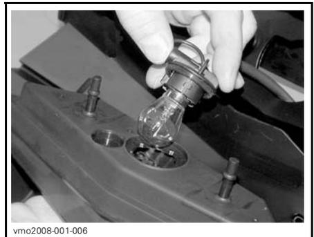
Push the bulb in and hold while turning counterclockwise to release.
