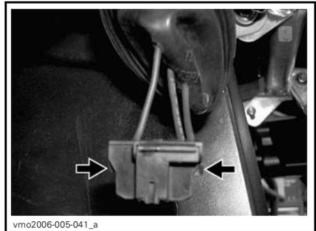
**PUSH ON LOCKING TAB TO UNLOCK CONNECTOR**
