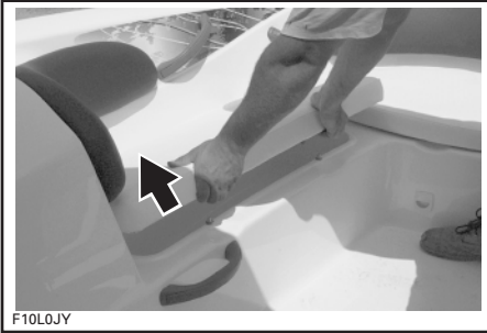
Step 1: Pull a small amount to unlatch Step 2: Gently rotate clockwise
