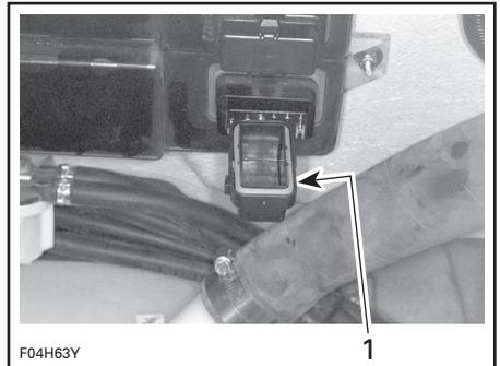
1. Slide cover tabs on each side of fuse then pull fuse out
