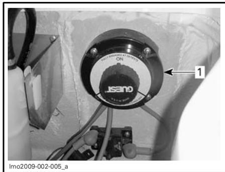
TYPICAL — MAIN BATTERY CUT-OFF SWITCH
