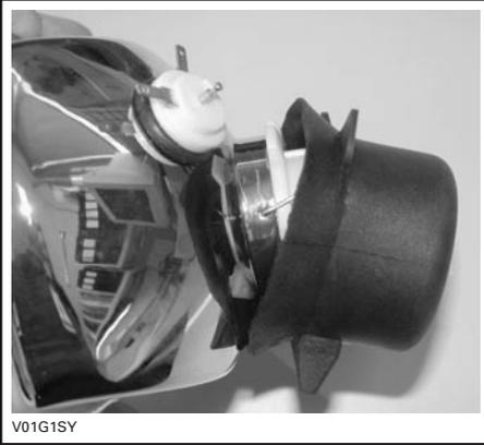
Unlock the bulb socket.
