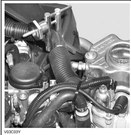
Fill the radiator until the coolant comes out by the thermostat housing hole. Install the bleeding screw then remove the hose pincher.
