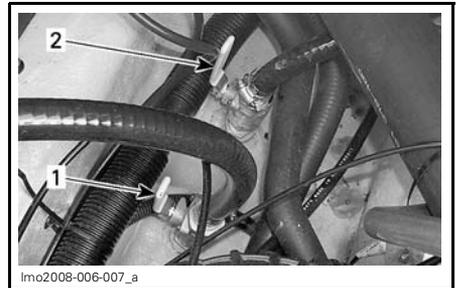
**THRU-HULL VALVES — OPEN POSITION**
