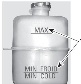
1. Level between marks when engine is cold B00067
