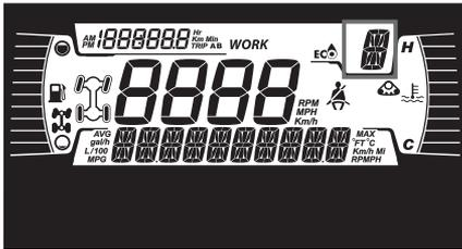
This display shows gear position of gearbox:
