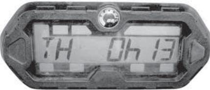
Press and HOLD the selector button for 2 seconds to reset the hour meter.
