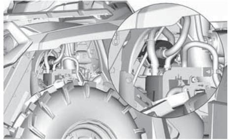
1. Cut the locking tie securing the round filter on the top of the EVAP canister support.
