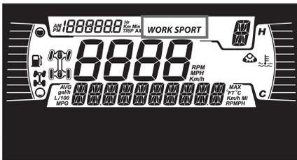
The MODE display indicates the selected mode of operation:
