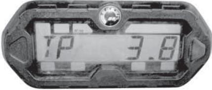
Press and HOLD the selector button for 2 seconds to reset the trip meter.
