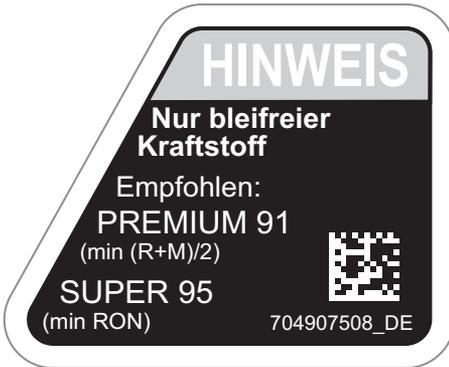
1000R-MOTOREN - IN DER NÄHE DES KRAFTSTOFFTANKDECKELS
